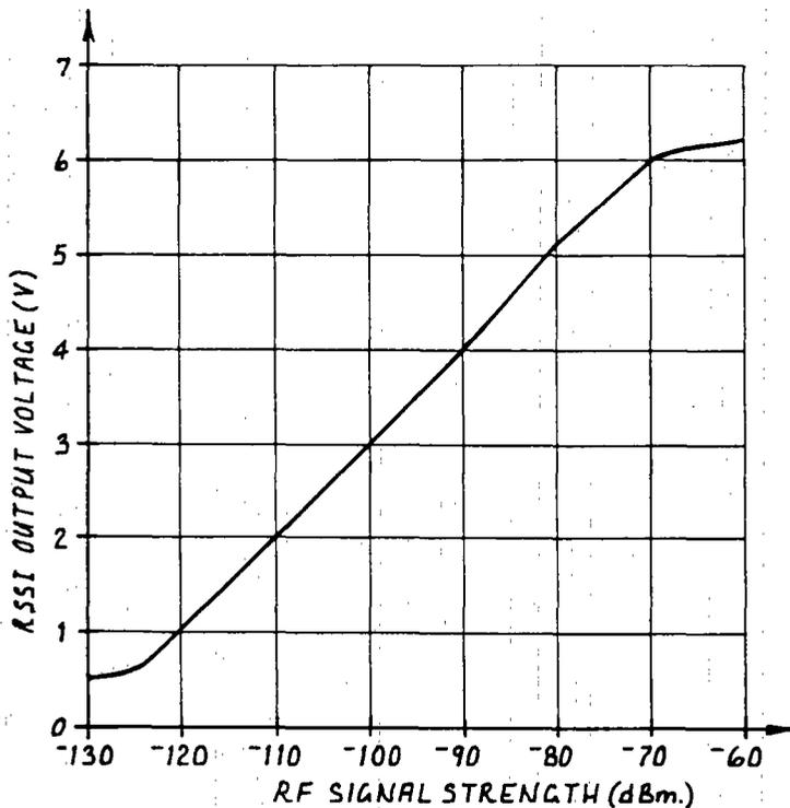
Figure 24 RSSI Voltage vs Signal Strength
