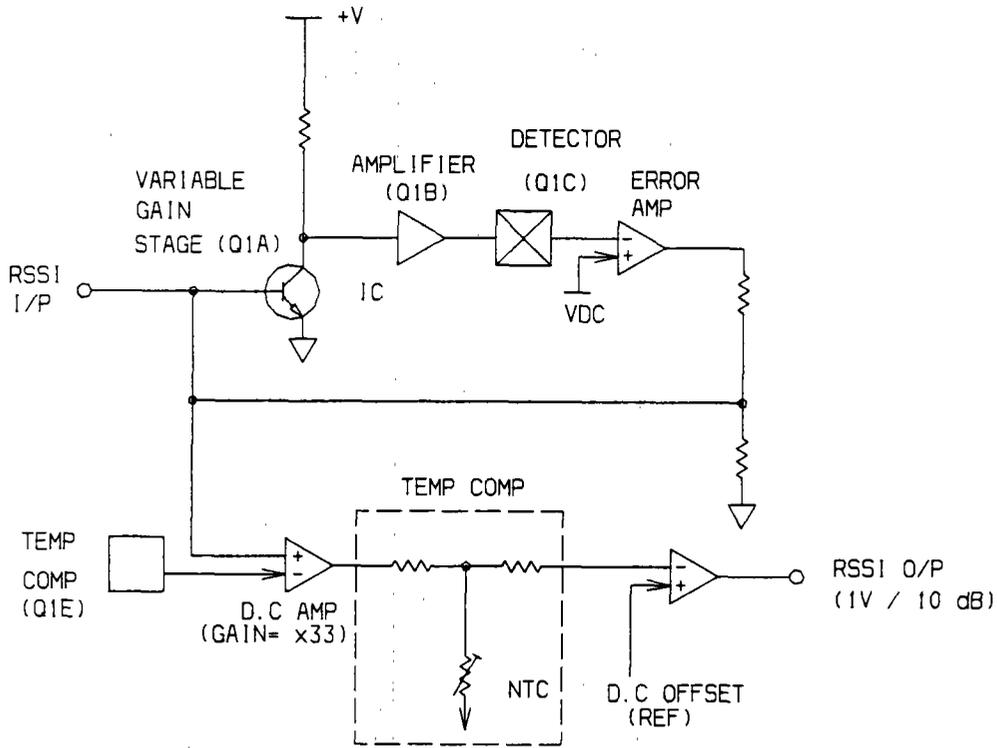
Figure 6 RSSI Block Diagram
