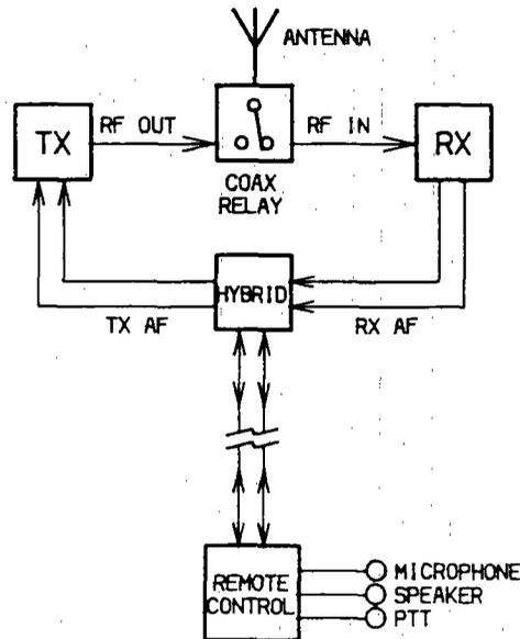
Figure 18 Remote Line Controlled Base Station
