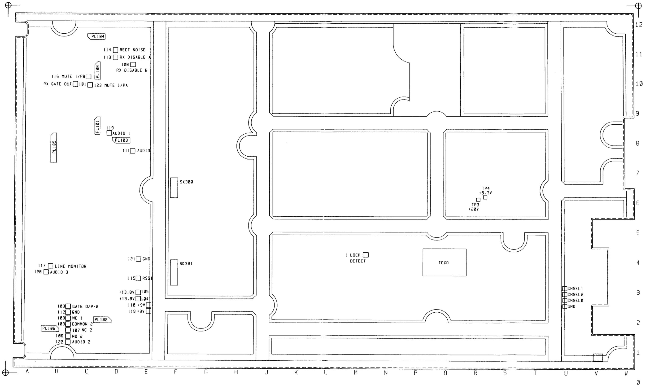
DIAGRAM 7 - T885 TESTPOINTS AND OPTIONS - TOP SIDE.
