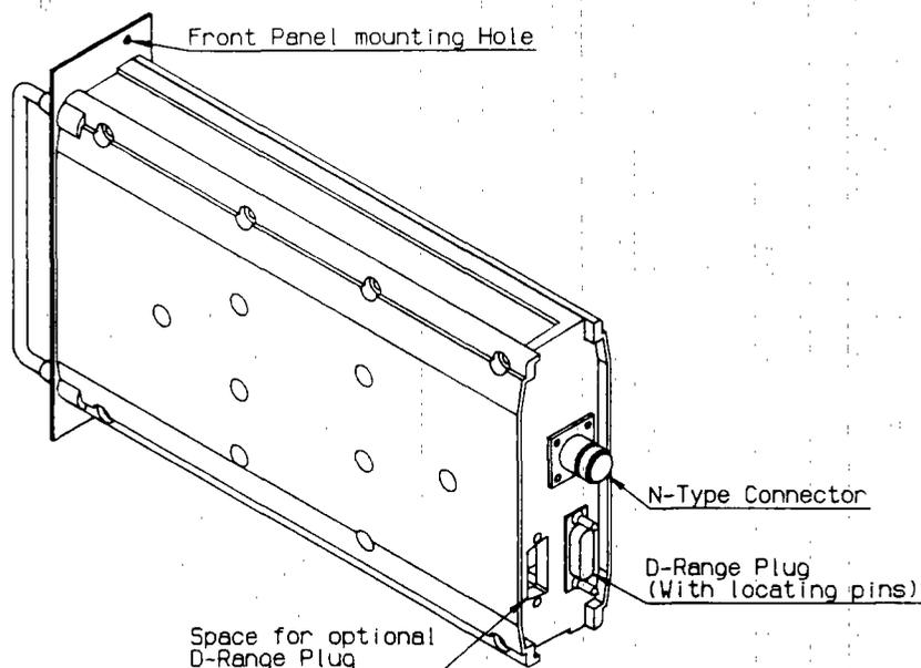
Figure 14 T885 Chassis Connectors
