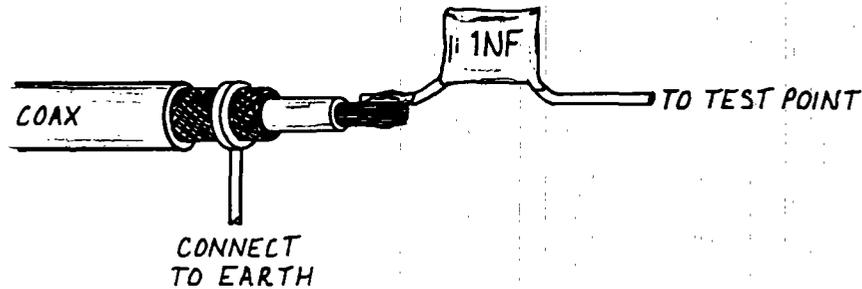
Figure 10 RF Test Cable
