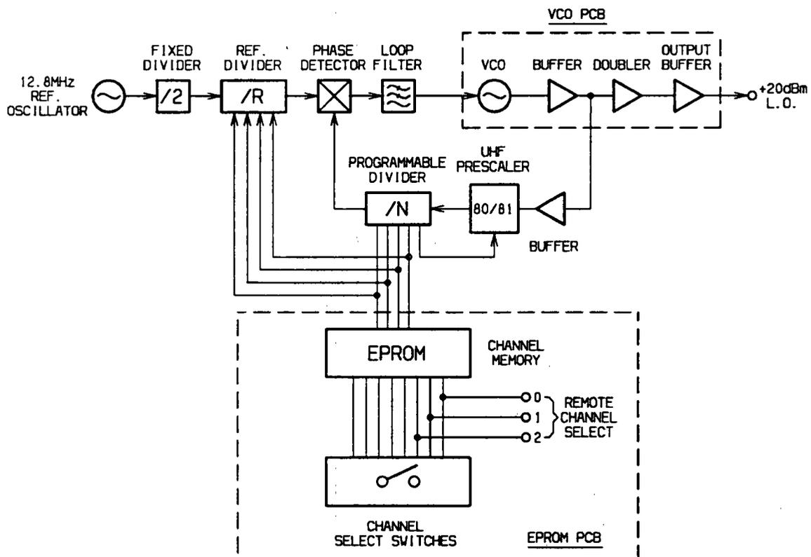
Figure 5 Synthesiser Block Diagram
