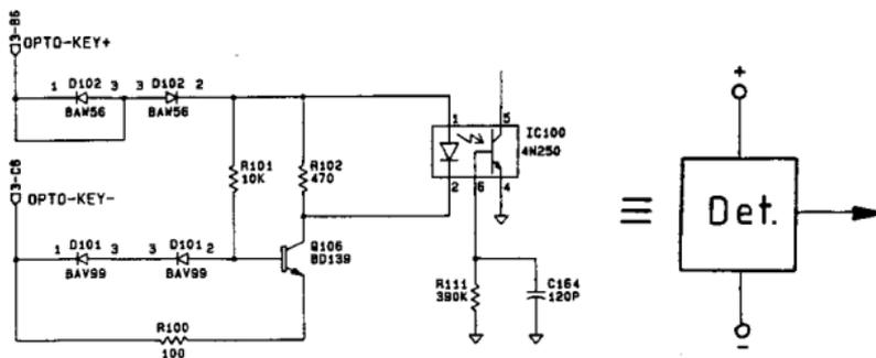
Figure 21 Isolated Constant Current Loop Current Detector
