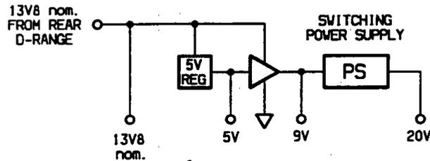
Figure 4 Power Supply and Regulator Block Diagram
