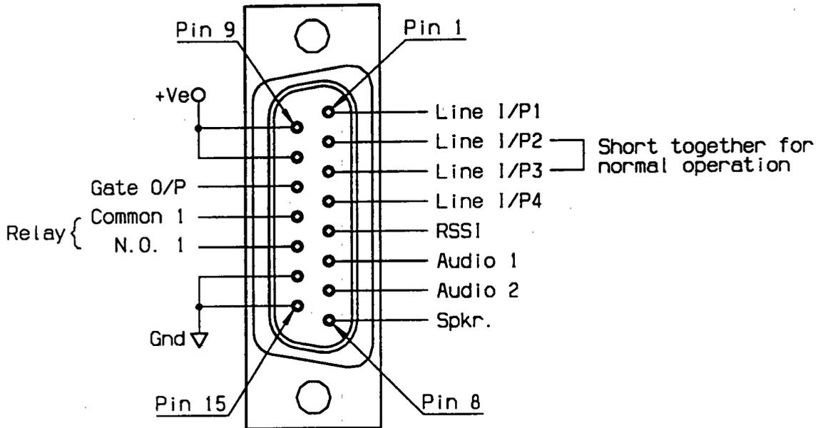
Figure 15 D-Range Wiring - Rear View
