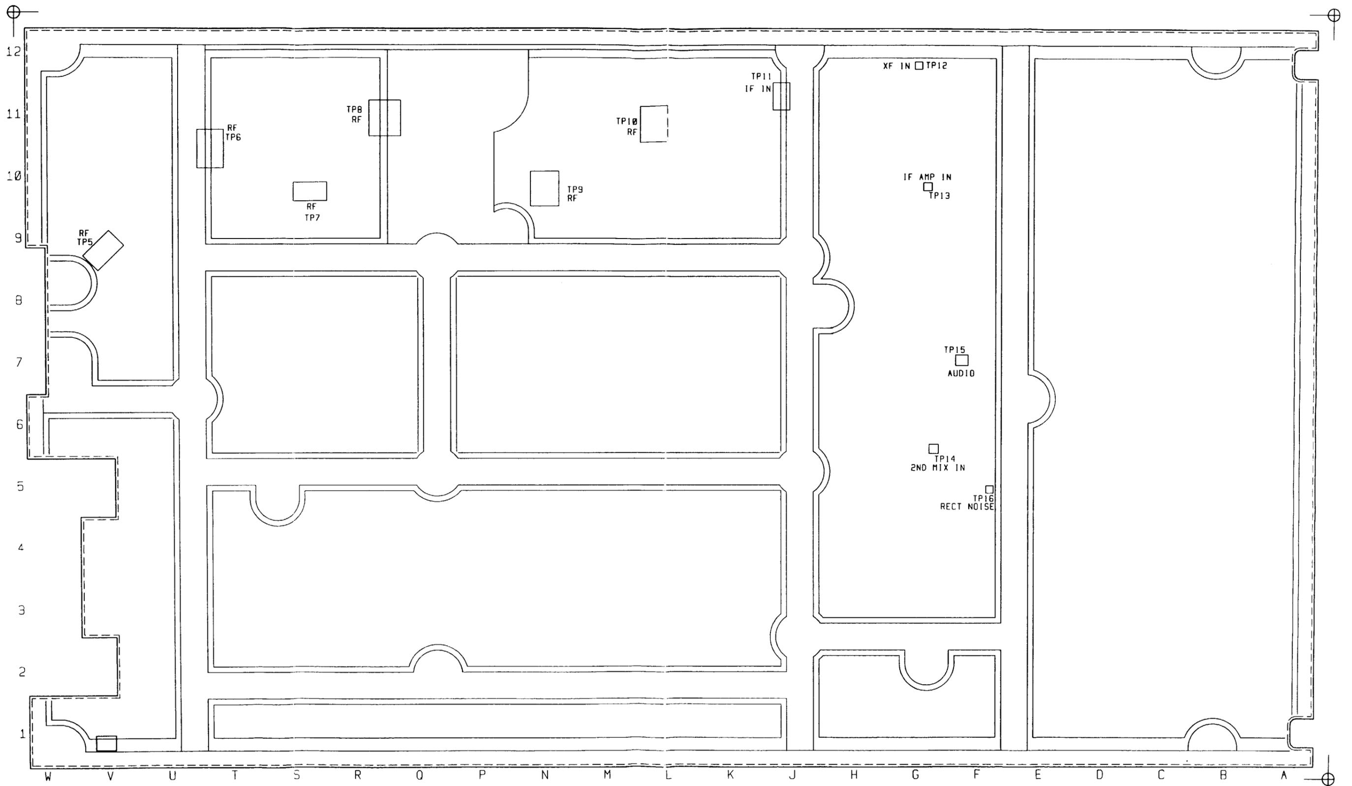
DIAGRAM 8 T885 TEST POINTS AND OPTIONS - BOTTOM SIDE.
