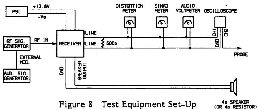
Figure 8 Test Equipment Set-Up
