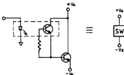
Figure 22 Isolated Loop Current Switch
