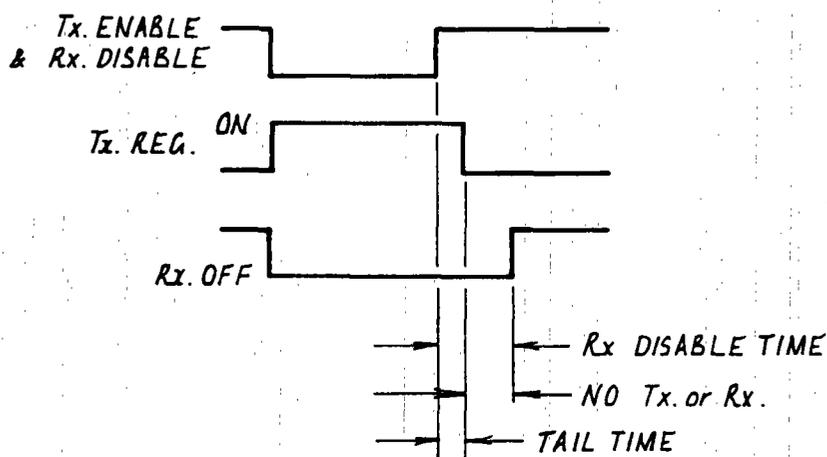
Figure 19 Receiver Disable Time vs Tail Time
