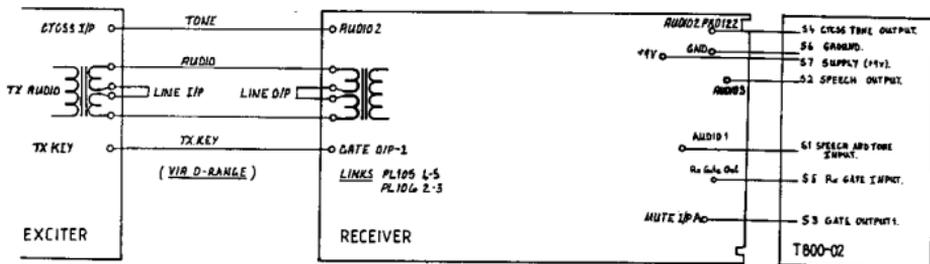
Figure 26 CTCSS Wiring Detail
