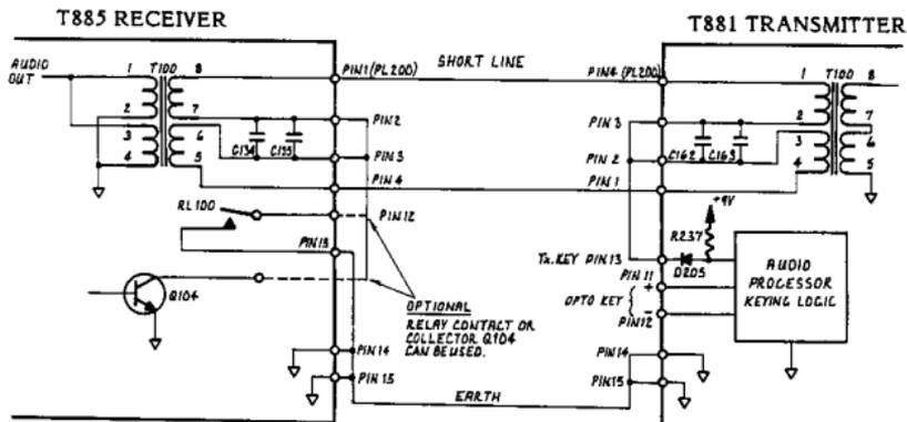
Figure 20 DC Loop Keying With Common Earth
