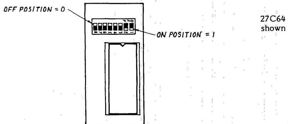
Figure 7 Channel DIP Switch Setting
