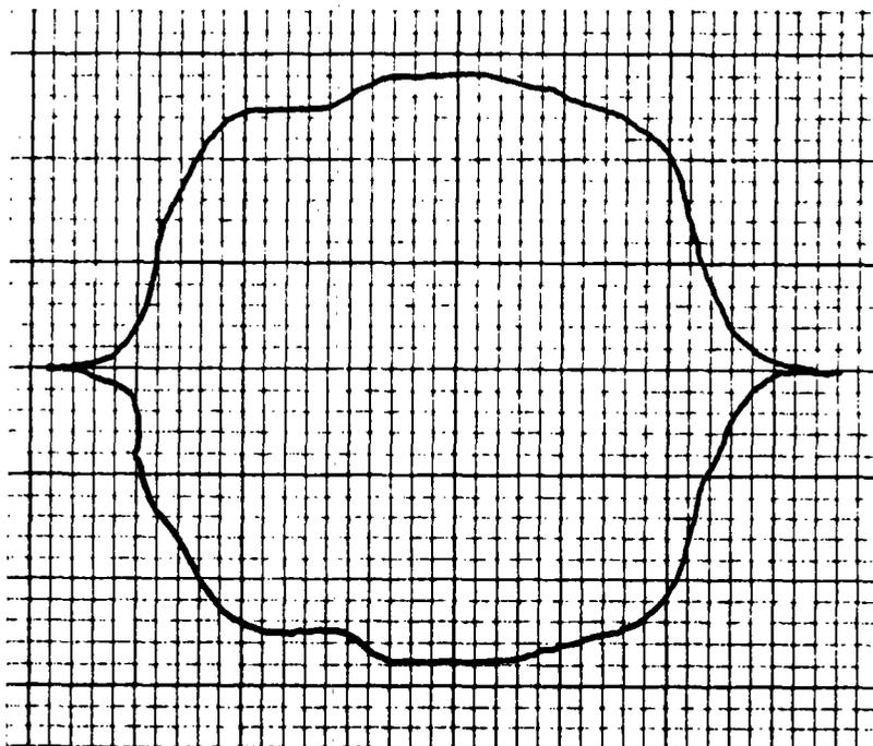
Figure 12 Ceramic Filter Swept Response
